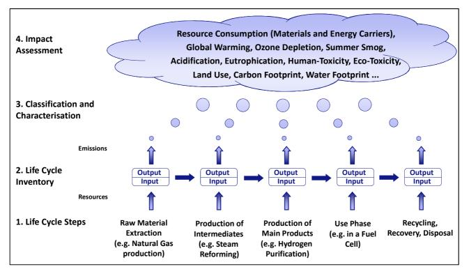
Figure 1: Overview of the LCA methodology
