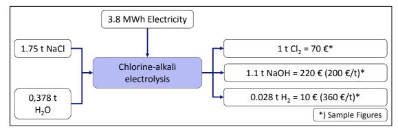
Figure 7: Sample products of chlorine-alkali electrolysis with sample prices
