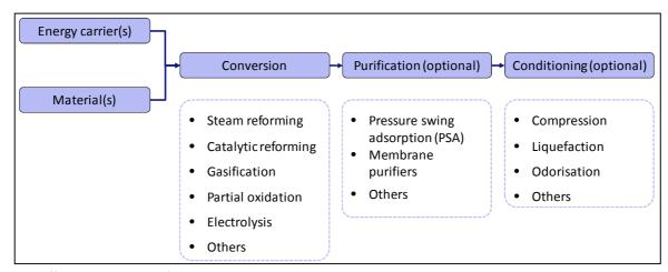
Figure 3: Different pathways of hydrogen production
